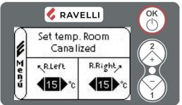
Confirm with the OK button twice until the screen for setting the room temperature set for the two ducted rooms appears.
