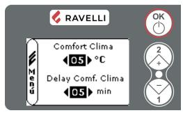
The activation of this function enables the stove to reduce pellet consumption by activating the modulation phases, after the desired temperature has been reached. Subsequently, the stove checks that the temperature is maintained steady for a preset time (DELAY COMFORT CLIMA). If this condition is met, it automatically switches off, and on display appears the writing ECO STOP. The stove turns on again when the temperature drops below the set threshold (COMFORT CLIMA).
