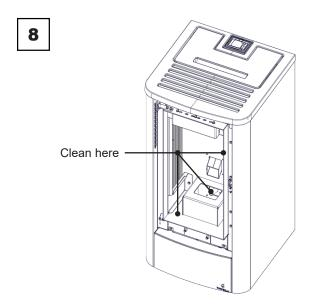
After cleaning the combustion chamber, it is advisable to proceed with the cleaning of the inspection hatches as indicated in the paragraph "Smoke duct cleaning".
