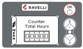
You can see the working hours of the stove. To scroll the different counters (total or partial hours and number of ignitions) use key 1 and 2.
