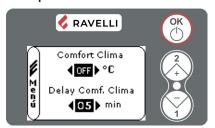
To activate the function, set the COMFORT CLIMA value different from OFF using buttons 1 and 2. Confirm with OK.
