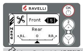
The upper part of the display allows you to change the power of the front ventilation. The settable value ranges from 0 (fan off) to 5. With setting on A (auto) the power of the fans follows the power of the stove.
