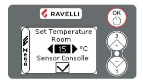
Set the desired temperature with keys 1 and 2. The selectable values are: EST, from 7 °C to 40 °C (or from 44 °F to 104 °F), MAN. The EST value must be selected if you want to use the external thermostat and MAN when you want to make the stove work at constant power.
