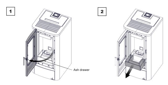
Vacuum the residues present in the ash compartment with a suitable ash vacuum cleaner, making sure that the ashes are completely extinguished.
